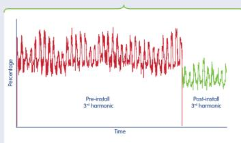
The **powerPerfector** is able to deliver significant reductions to the 3<sup>rd</sup>, 5<sup>th</sup> and 7<sup>th</sup> order harmonics. It reduces currents flowing on the neutral by attenuating triple-n harmonics, and helps to balance the three phases supplied to your site.
